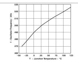
Figure 1. Oscillator Frequency vs. Junction Temperature
