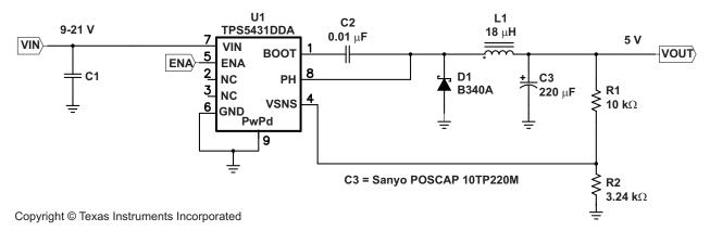
Figure 18. 9 V – 21 V Input to 5 V Output Application Circuit
