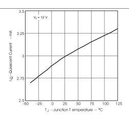
Figure 2. Non-Switching Quiescent Current vs. Junction Temperature
