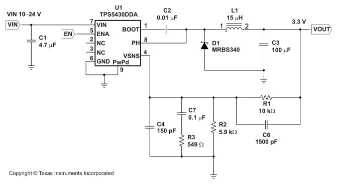
Figure 19. Ceramic Output Filter Capacitors Circuit
