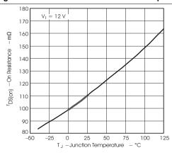
Figure 5. On Resistance vs. Junction Temperature
