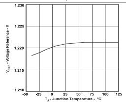
Figure 4. Voltage Reference vs. Junction Temperature
