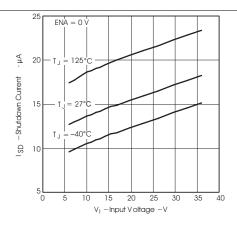
Figure 3. Shutdown Quiescent Current vs. Input Voltage
