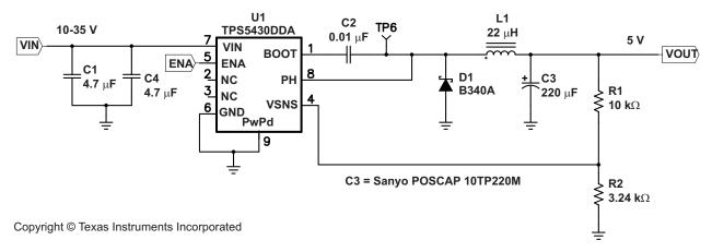
Figure 17. 10 V-35 V Input to 5 V Output Application Circuit
