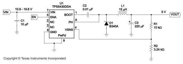
Figure 9. Application Circuit, 12 V Input to 5.0 V Output
