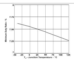
Figure 8. Minimum Controllable Duty Ratio vs. Junction Temperature
